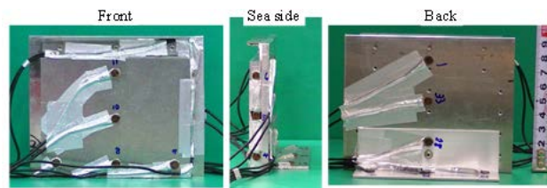
Fig. 8. Pressure sensors placed on the abutment of conventional type bridge model.
